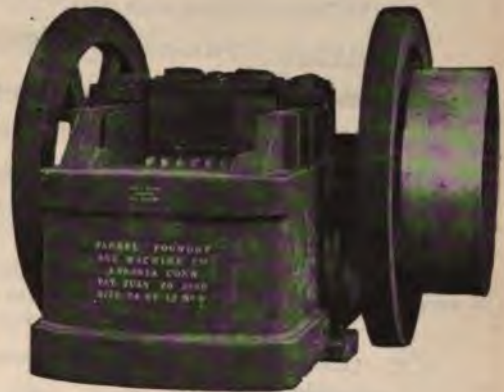
FARREL Ore and Rock Crusher.
